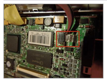
Use <u>tweezers</u> to remove last piece from the comb on the motherboard.
