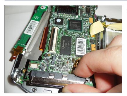
Remove the motherboard by simply lifting it.
