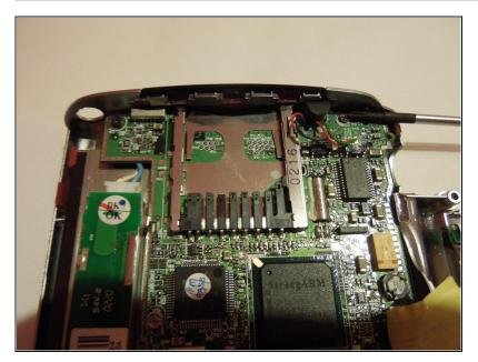
Remove the two screws on top of the motherboard and the two screws on bottom of motherboard
