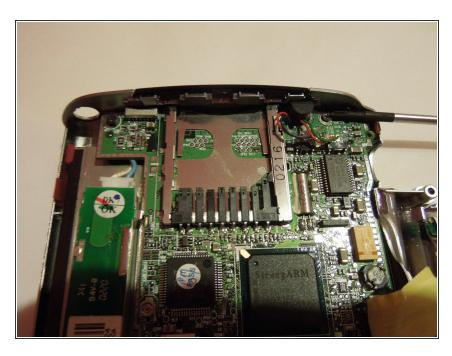
Remove the two screws on top of the motherboard and the two screws on bottom of motherboard
