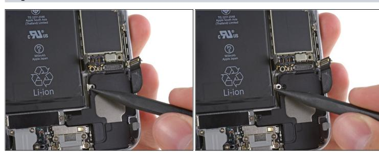
Use the point of a spudger to push the antenna interconnect cable clip off of the speaker housing.
