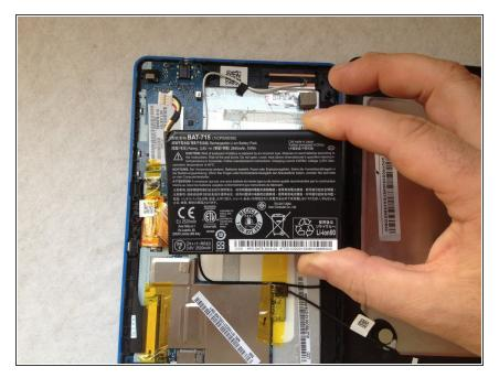
• Li-on Batteri Pack, 3.8V, 2640mAh
