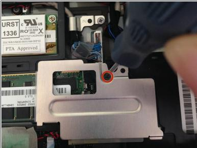
Using a #00 philips head screwdriver, remove the 6mm screw holding the metal plate down.
