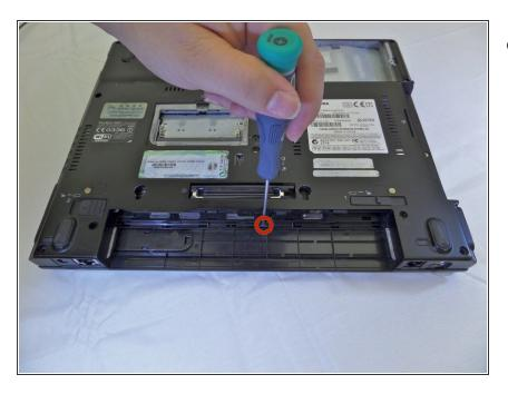
Use a #00 phillips head screwdriver to remove the 8mm screw for the keyboard strip located under the battery.
