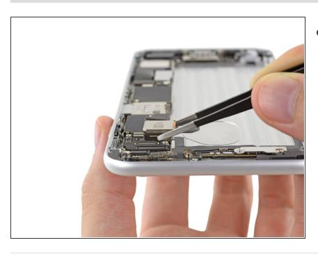
Carefully lift and remove the rearfacing camera out of the iPhone.
