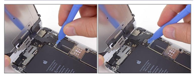
⚠ In the next four steps, take care to pry up **only** on the cable connectors, and not on their sockets on the logic board.
