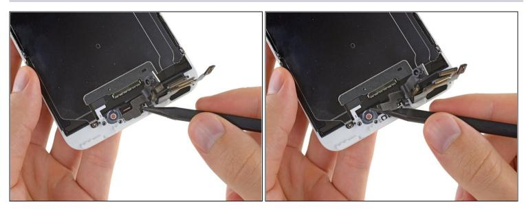
• Use the tip of a spudger to gently pry up the sensor cable assembly from its recess in the display assembly.
