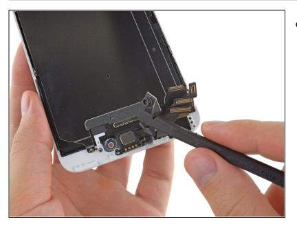
• Use a the flat end of a spudger to pry up the front-facing camera and display cables, and gently push them aside.
