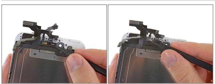
• Pry the microphone portion of the front-facing camera and sensor cables from the display assembly.
