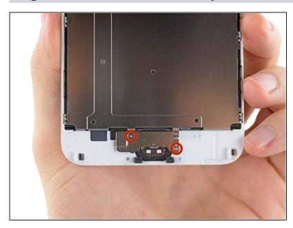
Remove the two 1.8 mm Phillips screws securing the home button bracket to the front panel.
