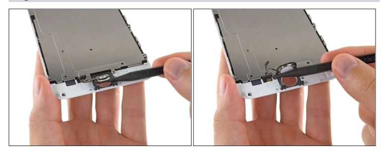
• Carefully use the tip of a spudger to finish separating the home button from the front panel.
