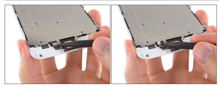
• Use the tip of a spudger to disconnect the home button connector from its socket on the home button cable.
