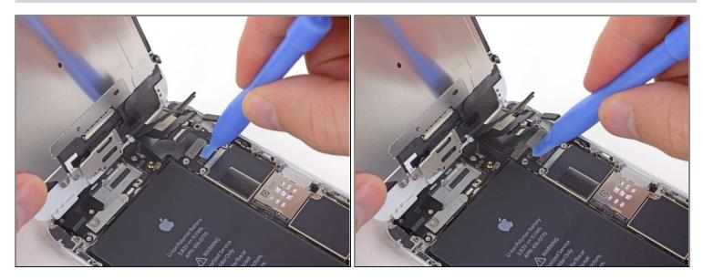
A Make sure the battery is disconnected before you disconnect or reconnect the cable in this step.
