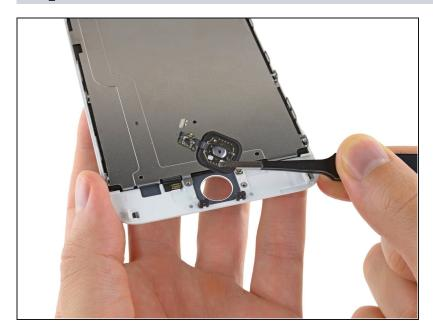
• Lift and remove the home button assembly off the front panel assembly.
