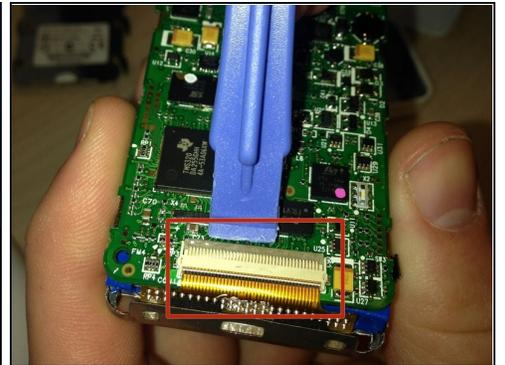
⚠ Do not damage the ribbon tab (pictured). It is vital to the device.
