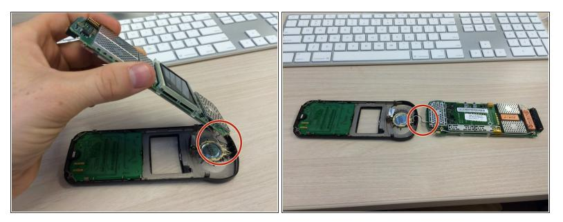
• Flip the motherboard over so that the screen is facing down.
