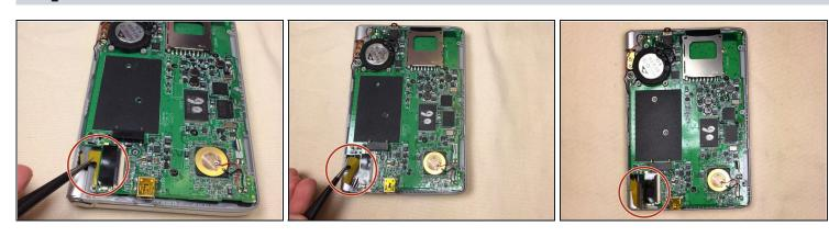
• Using a pair of <u>tweezers</u>, pinch the center of the yellow ribbon located in the corner of the device.
