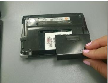
• Place your fingers on the battery cover arrow and pull the cover down and off the device.
