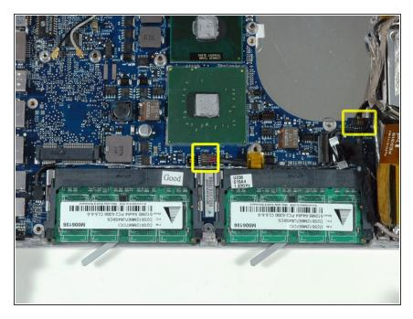
Use a spudger to disconnect the two speaker connectors from the logic board.
