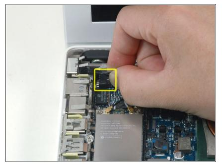
• Disconnect the MagSafe board cable from the logic board.
