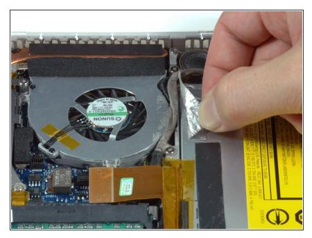
• Peel up the foil tape between the fan and the optical drive.
