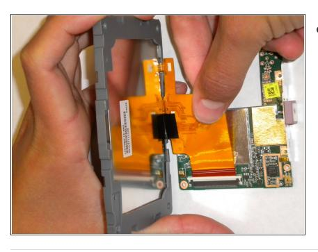
Remove the motherboard from the device.
