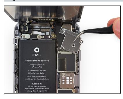
Remove the front panel assembly cable bracket from the logic board.
