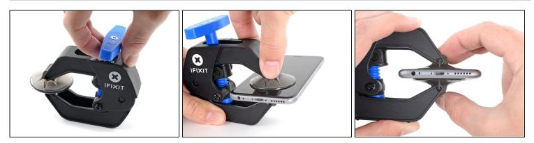
(i) The next two steps demonstrate the <u>Anti-Clamp</u>, a tool we designed to make the opening procedure easier. If you aren't using the Anti-Clamp, skip down three steps for an alternate method.
