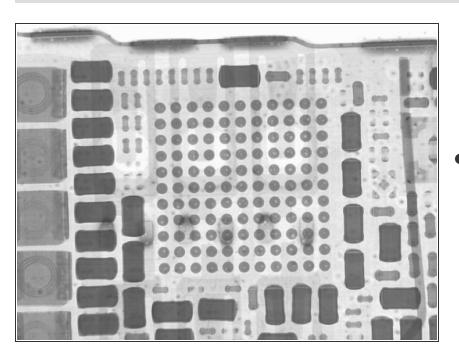
We know voids in ball grid arrays (BGA) can be problematic to the reliability of any electronic product. In our x-ray inspection of the iPhone 5S, we noticed that the Apple 338S120L chipset had a large number of voids. So the natural next step was to use the BGA inspector included in the TruView 200 to measure the voids.
