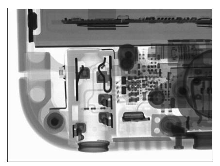
This corner shot of the iPhone 5S shows the standard 3.5mm audio jack. You can also see the corner of the Touch ID interface and supporting mechanics.
