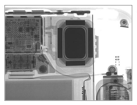
This corner of the iPhone 5S has not changed since the iPhone 5/4S. The large high performance speaker is located in the same place, and the antennae connections are very similar to previous models.
