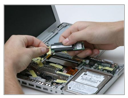
• Disconnect the modem cable from the modem.
