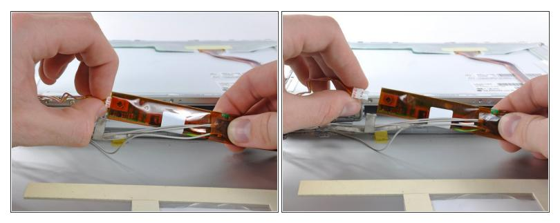
• Disconnect the inverter cable by pulling the connector away from the socket on the inverter board.
