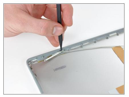
Place the pointed end of the spudger behind the lower part of the antenna and carefully rotate the spudger to free the antenna from the rear display bezel.
