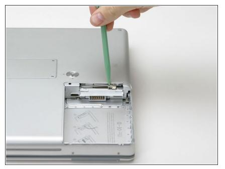
• Use a spudger to disconnect the Airport antenna from the card.
