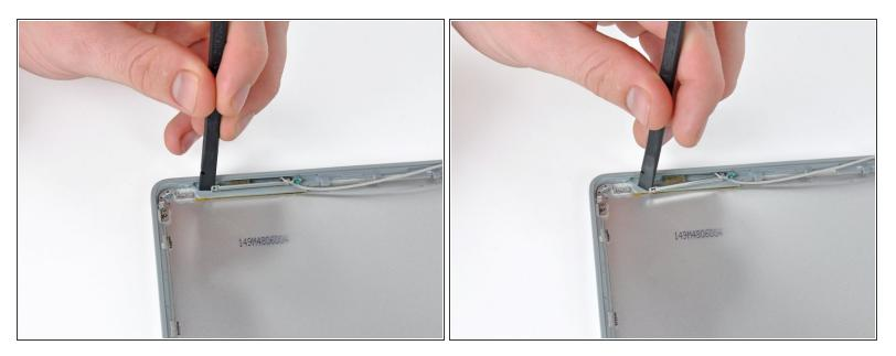
The antenna is attached to the rear display bezel via adhesive. To remove it, place the flat end of a spudger behind the top edge of the antenna, and carefully twist the spudger to pop the antenna off.
