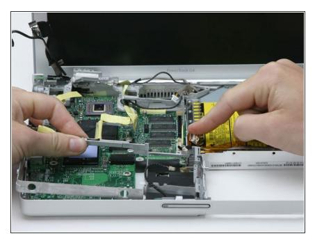
• Lift the metal framework out of the computer. Be careful that the orange optical drive cable doesn't catch on the framework and be sure you haven't forgotten to disconnect any other connectors.
