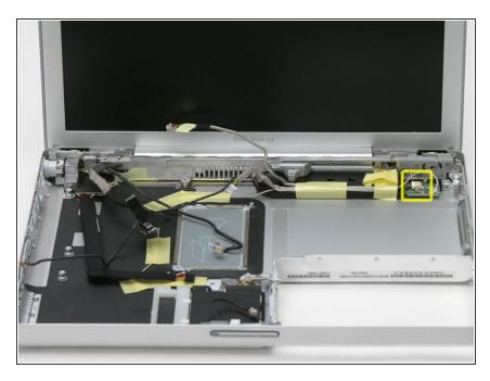
• Disconnect the multicolor connector by sliding it to the left.
