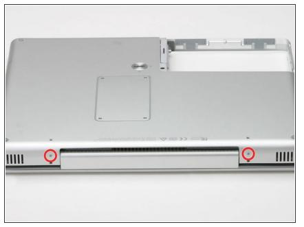
• Remove the two Phillips screws from either side of the display hinge.
