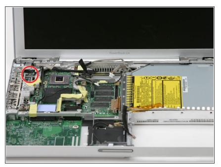
• Remove the single Phillips screw from the RJ-11 board.
