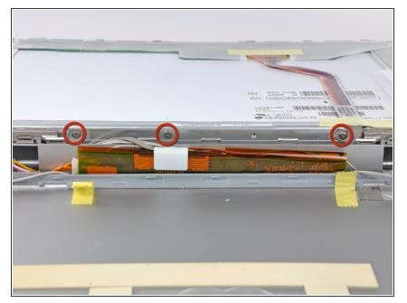
Remove the three 3.0 mm Phillips screws connecting the clutch cover to the front display bezel.
