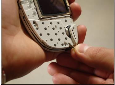
• Remove the six Torx T6 screws from the phone's front case.
