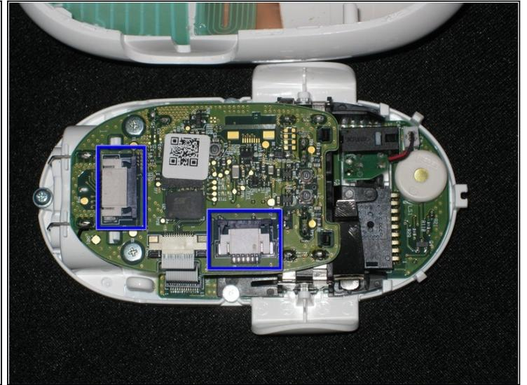
⚠ Gently unlock the latches with a fingernail or a spudger. Do not stress the latch, or it might break.
