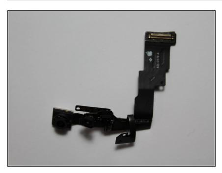
The front camera and proximity sensor flex cable.
