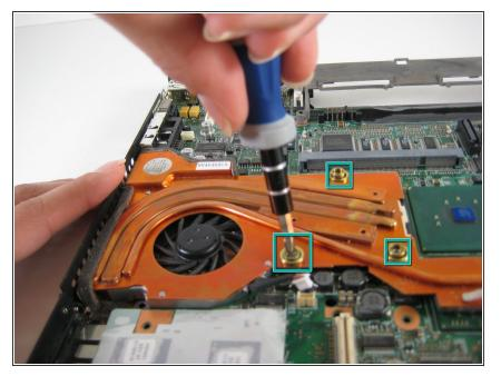
• Remove the three screws on the fan.
