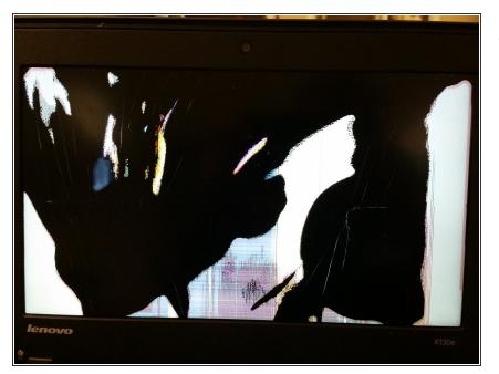
Before ordering a new LCD, determine if the old one is cracked or damaged. If it is damaged, power off the machine and remove the battery.
