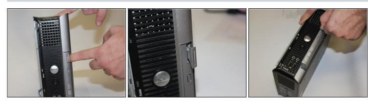
Press the large button on the corner of the optical drive. Pull on the pop-out button to slide the optical drive out.
