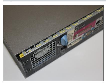
While the knob is still turned, slide the panel case forward about 1/2 inch, and then lift the panel off the computer.
