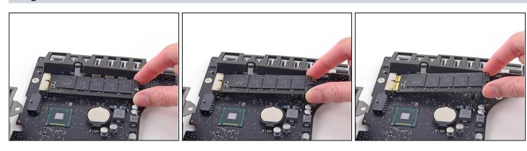
• Slightly lift the rightmost side of the SSD and firmly slide it straight away out of its socket on the logic board.
