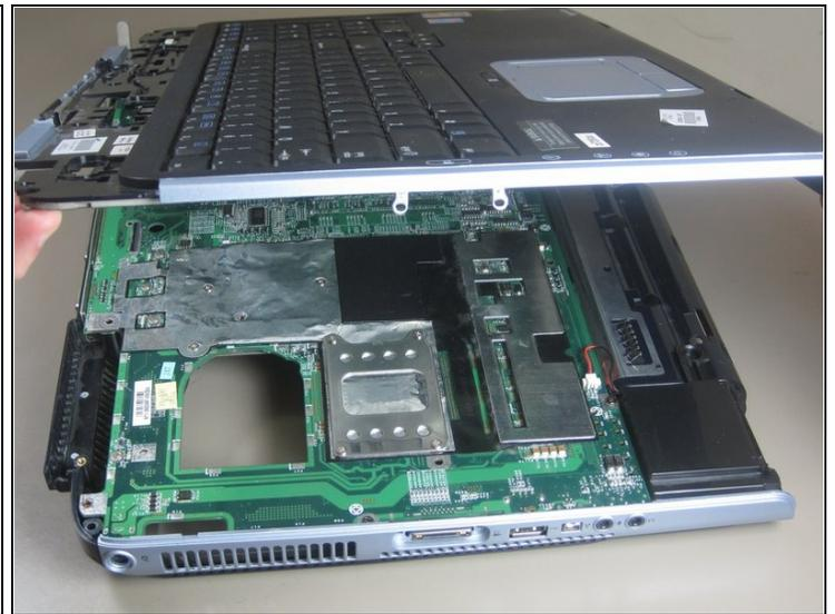
**⚠ Do not remove the keyboard yet! There are still wires connecting the two components.**
