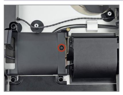
• Remove the single 7.2 mm T10 screw securing the hard drive tray to the rear enclosure.
