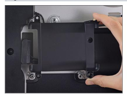
• Remove the hard drive tray from the rear enclosure.
