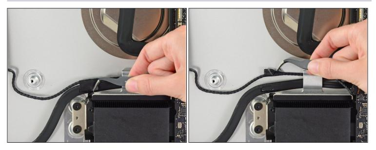
• If necessary, use a pair of <u>tweezers</u> to gently peel the tape securing the left speaker cable to the SATA data/power cable.
