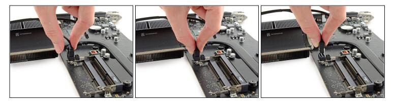
(i) The SATA data connector has a clip that must be pressed to allow removal.
