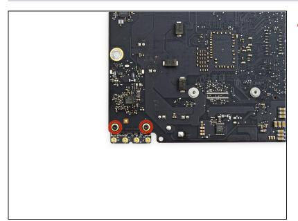
Remove the two 3.2 mm T5 screws securing the AirPort/Bluetooth card to the logic board.
