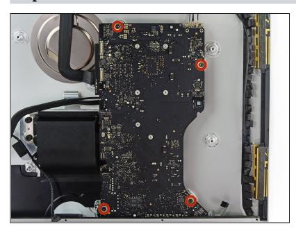
Remove the four 7.2 mm T10 screws securing the logic board to the rear enclosure.
