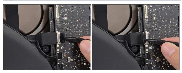
• Use the tip of a spudger to flip up the metal retaining bracket on the iSight camera cable located on the logic board.
