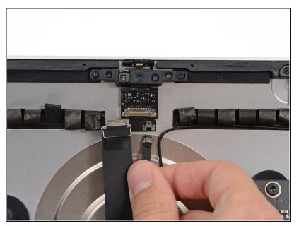
Disconnect the microphone cable from its socket on the camera board by carefully pulling straight down.
