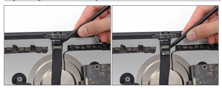
• Use the tip of a spudger to flip down the metal retaining bracket on the iSight camera cable.
