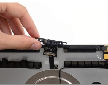
Lift and remove the camera assembly from the iMac.
