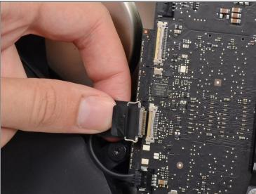
• Pull the iSight camera cable straight away from its connector on the logic board.
