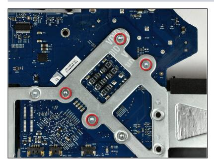
Remove the four fine-thread 5 mm T8 Torx screws securing the heat sink to the logic board.
