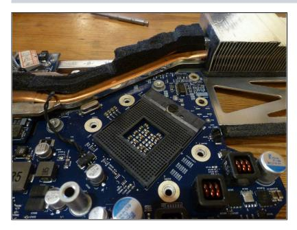
remove the CPU. Be careful, don't bend the pins!
