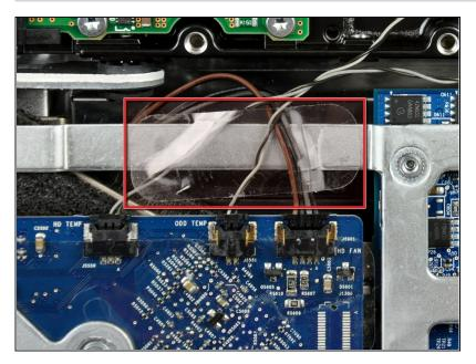
If necessary, remove the piece of tape securing the thermal sensor and fan cables to the chassis.
