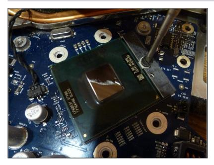
turn the black "screw" an half turn counter clockwise to unlock the CPU
