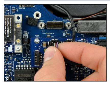
Pull the right speaker cable connector straight up out of its socket on the audio board.
