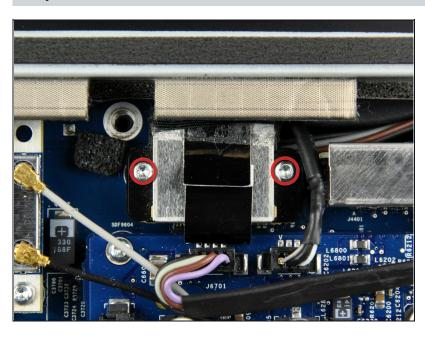
Remove the two 5.3 mm T6 Torx screws securing the data display cable to the logic board.
