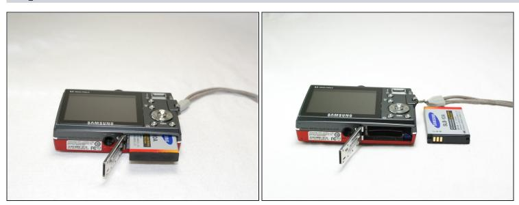
• Open the battery cover that's located on the bottom right side of the camera and carefully remove the battery.
