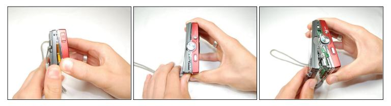
• Slide your fingernail or a plastic spudger in the groove from the bottom to the top right side of the camera.
