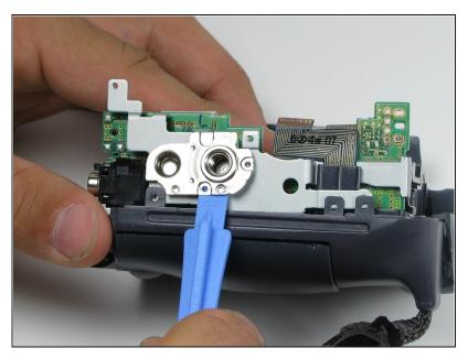
Remove tripod mount carefully by prying it off with a plastic opening tool.
