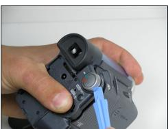
Locate the blue plastic tool opener, then remove both the round record/playback and record/power control knobs by prying it open from the camcorder.
