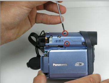
Remove the indicated 4.5mm screws from the LCD side of the camera.
