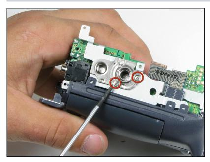
Remove two 4.5mm silver tripod mount screws.
