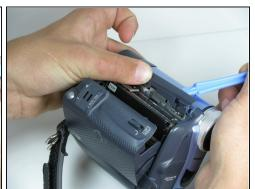
• Use the blue plastic opening tool to remove the gray trim piece by prying it from top of the camcorder.
