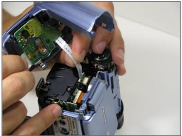
Using your fingers, carefully pull the ribbon cable away from the logic board.
