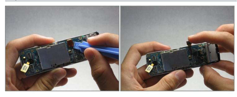
Use the iFixit opening tool to remove the other orange tab to free the motherboard.
