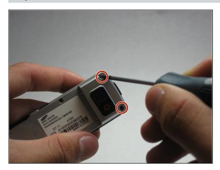
Remove the two 7.3 mm screws from the camera and the speaker at the bottom back plate of the phone using a Phillips #00 screwdriver.
