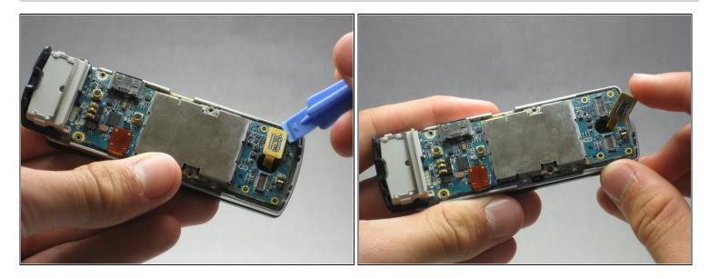
Use the iFixit opening tool to remove the yellow tab on the motherboard.
