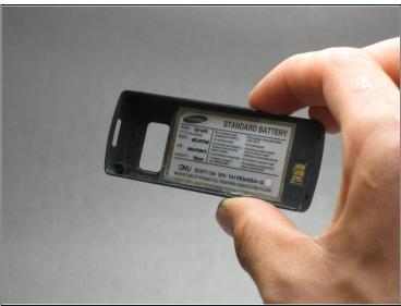
While holding the button down, remove the back cover of the phone.
