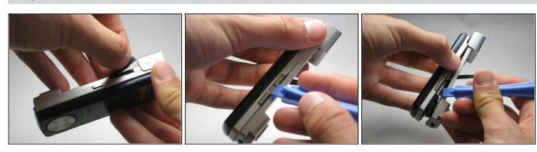
• Locate the USB port (where the charger can be plugged in). Using the iFixit opening tool, open the phone cover.
