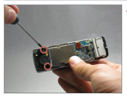
Remove the 5.5 mm screws from both sides of the camera/speaker with a Phillips #00 screwdriver.
