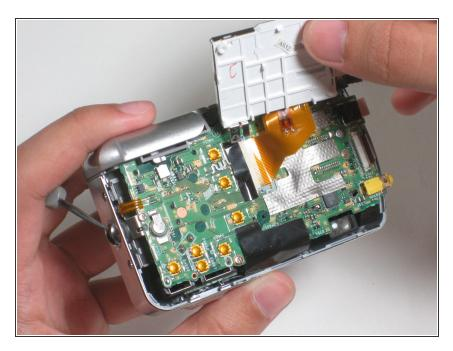
Carefully pull the LCD screen away from the board it is connected to.
