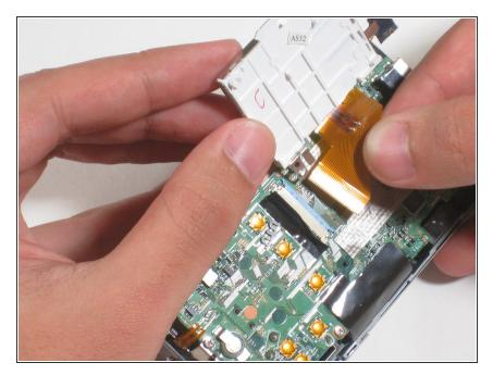
Carefully detach the ribbon from where it was connected by the blue pins.
