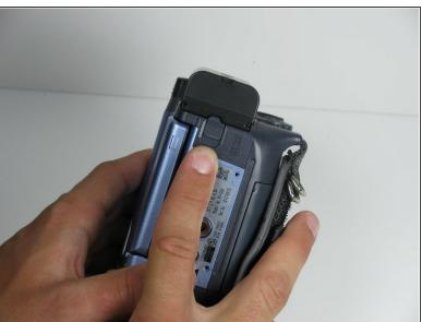
(i) While holding the Camcorder firmly, pull down on the battery removal tab located on the underside of the camcorder.
