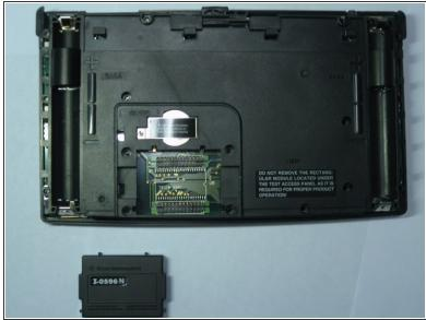
• Pull out the rectangular module when it is finally loose enough.
