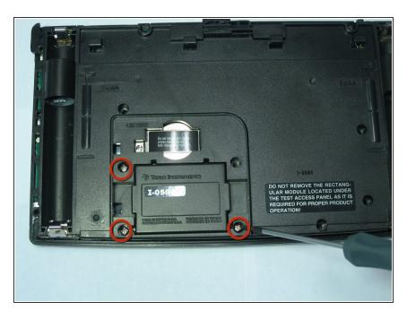
Using the same Phillips screwdriver, unscrew the remaining three
