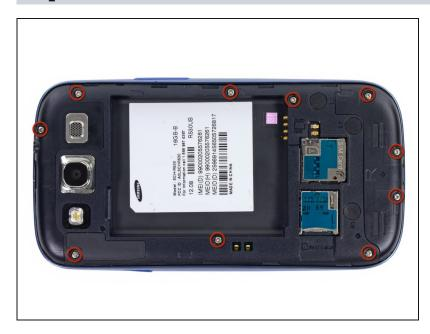
• Remove the ten 4.0 mm Phillips screws securing the midframe to the front panel assembly.
