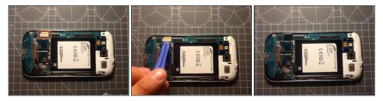
• Use the spudger to gently pry the display data cable from the motherboard.
