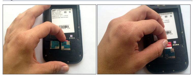
• If your provider/version of phone takes a SIM card, remove it by pushing it in a bit until you hear a small click, and then slide it out.
