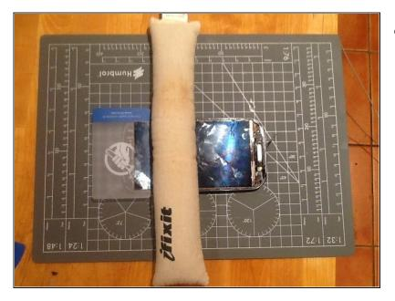
• As you work you will want to reheat the iOpener and put it back on the display to melt the adhesive further down the screen
