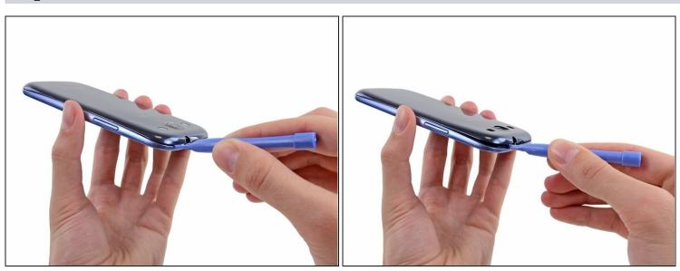
• Slide the plastic opening tool left along the top edge and repeat the twisting motion to widen the gap between the rear case and the phone.
