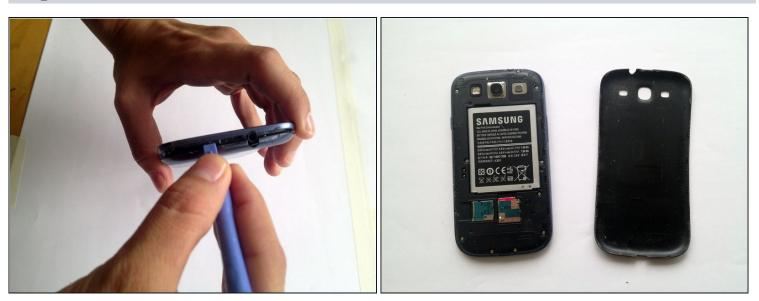
• With a plastic opening tool, pry open the back case. It will come out very easily.
