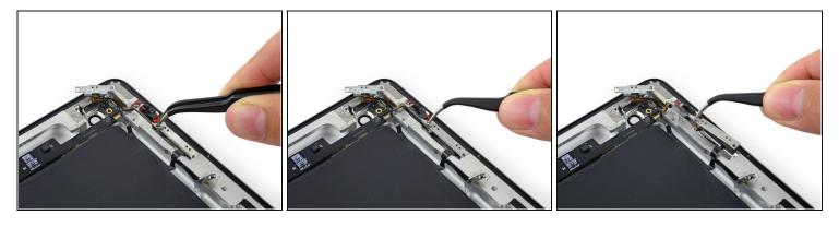
• Use the center screw hole of the volume control bracket to tilt it out toward the edge of the case and then pull it up out of its recess.
