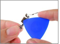
• Insert the point of an opening pick between the rotation lock/silent switch and its bracket to sever the adhesive there.
