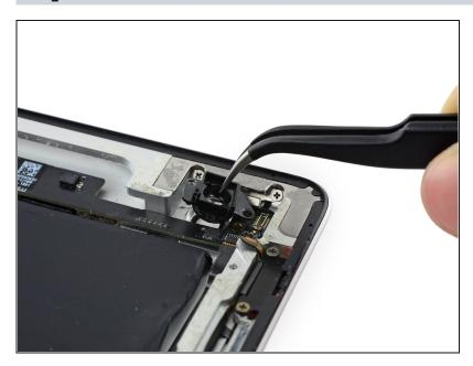
Remove the plastic camera bracket.
