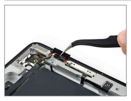
Remove the metal bracket securing the rotation lock/silent switch.
