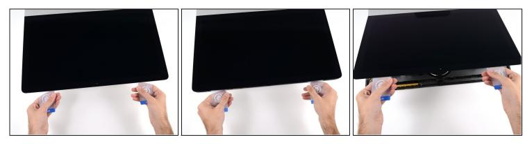
• With both plastic cards inserted as shown near the corners, gently twist the cards sideways to increase the gap between display and case.
