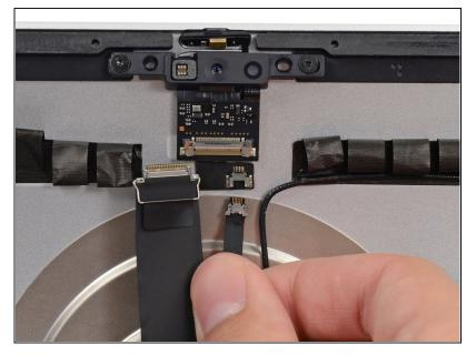
• Pull the microphone cable connector straight down out of its socket on the camera board.
