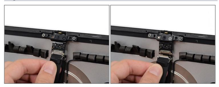
• Gently pull the iSight camera cable straight down and out of its socket on the camera board.
