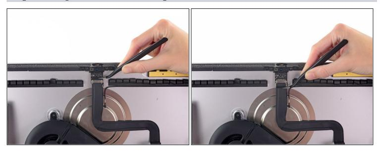
• Use a pair of tweezers to grasp and flip the metal retaining bracket downwards to free the iSight camera cable connector.
