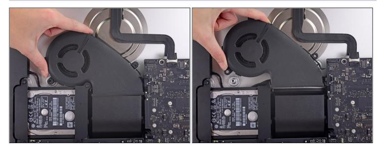
• Gently lift the fan up and remove it from the iMac.
