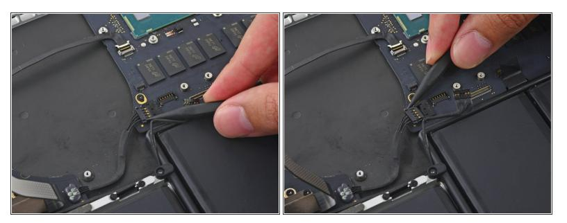
With the tip of a spudger, push on either side of the I/O board connector to walk it out of its socket on the logic board.
