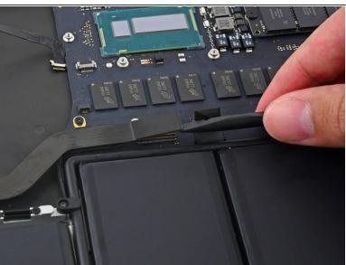
Use the flat end of a spudger to pop the I/O board connector straight up off its socket on the logic board.
