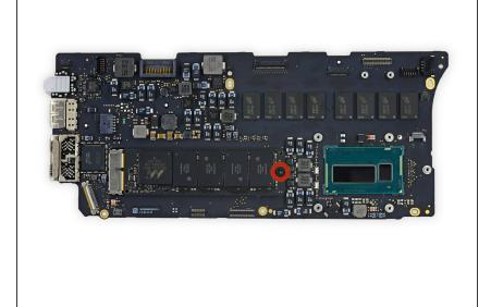
Remove the single 2.9 mm T5 Torx screw securing the SSD to the logic board.
