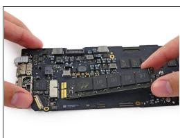
• Lift the free end of the SSD up slightly and pull it straight out of its socket on the logic board.
