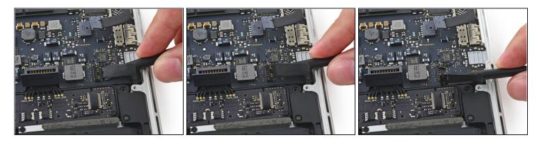
Wedge the flat end of a spudger under the left speaker cable near the connector and lift it straight up out of its socket and fold it out of the way.
