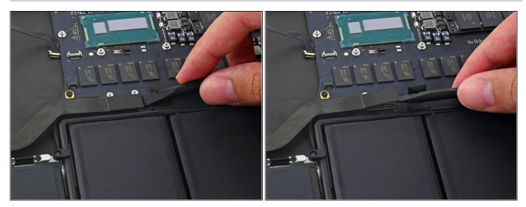
• Use the flat end of a spudger to pop the I/O board connector straight up off its socket on the logic board.
