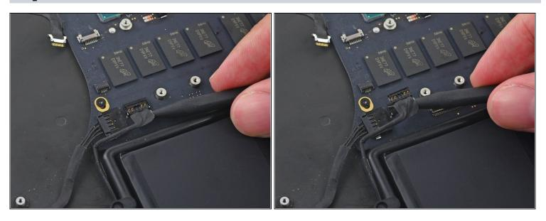
• Use the tip of a spudger to lift the right speaker connector straight up out of its socket on the logic board.
