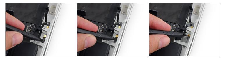
• Insert the tip of a spudger under the battery-side portion of the microphone ribbon cable and slide it toward the screw post to free it from the upper case.
