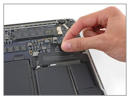
i If necessary, remove the plastic cover adhered to the battery contact board.
