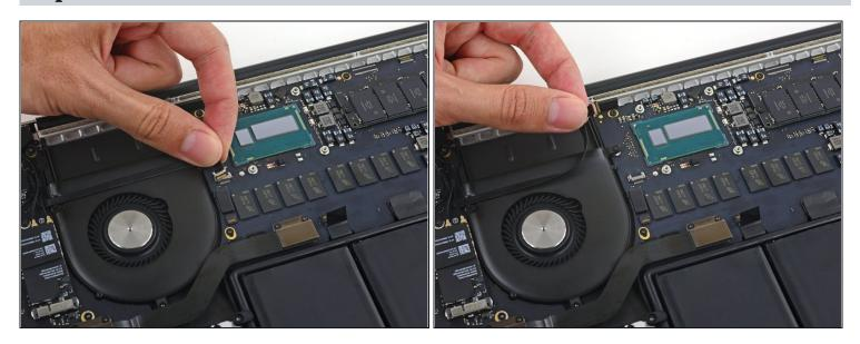
• Peel the iSight camera cable off the fan housing to fold it out of the way.
