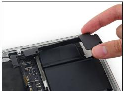
• Lift the corner of the left speaker up and slide it toward the battery to remove it from the upper case.
