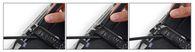
Remove the rubber microphone cover with a set of tweezers
