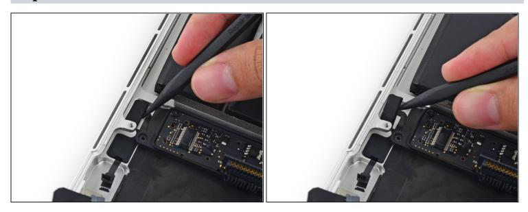
• Insert the tip of a spudger under the battery-side portion of the rubber microphone cable cover to detach the adhesive there.
