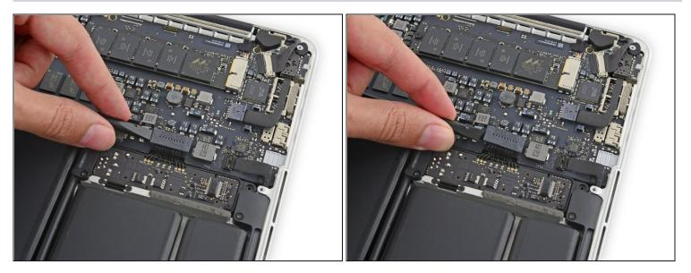
• Use the flat end of a spudger to lift the battery connector straight up out of its socket on the logic board.
