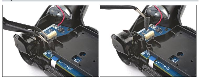
• Grab and remove the reset button extension from its recess in the battery bracket.
