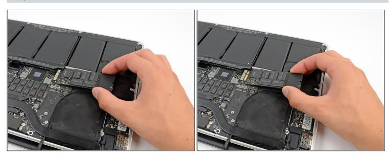
• Slightly lift the rightmost side of the SSD and firmly slide it straight away out of its socket on the logic board.
