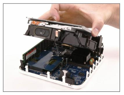
Grasp the optical drive and mass storage unit in one hand and lift up enough so that you can see beneath it.
