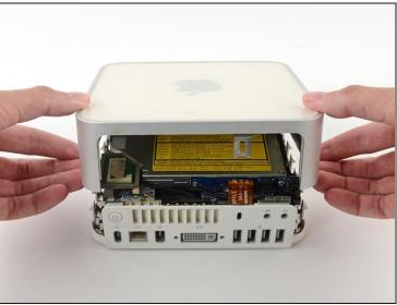
• Flip the Mac mini back over and lift the top housing off of the lower housing.
