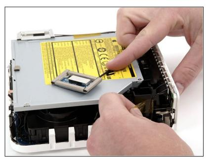
Remove the yellow tape securing the power button cable to the black plastic framework.
