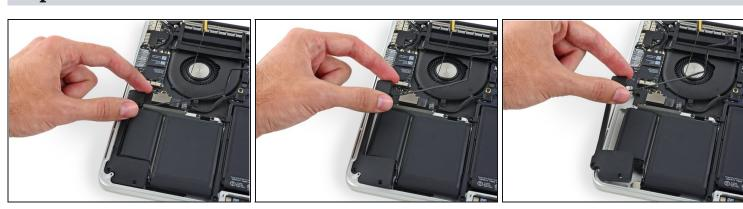
• Lift the right speaker from the cable end and pull it free from the case.
