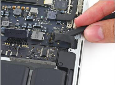
• Insert the tip of a spudger under the left speaker cable near the connector and lift it up out of its socket on the logic board.
