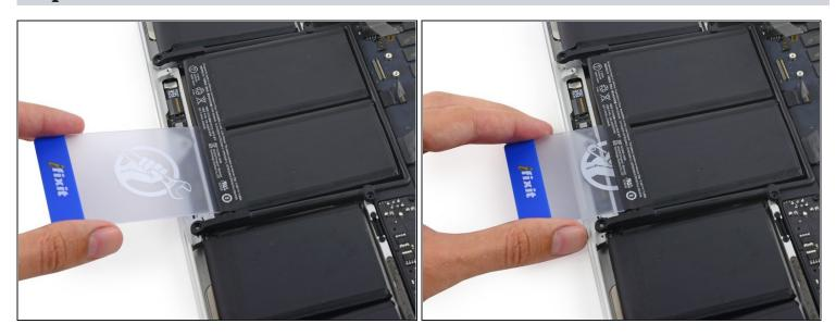
• Pull the card back out and insert it about an inch between the right-center battery cell and the upper case, separating the adhesive between the cell and case.
