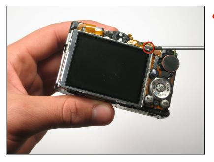
• Remove the screw at the upper right-hand corner of the LCD screen
