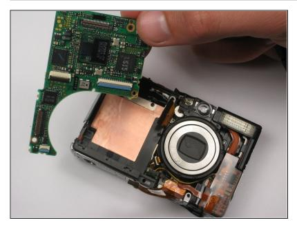
• Remove the detached logic board from the camera.
