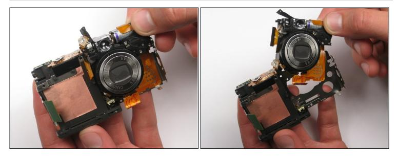
• Remove the lens carefully from the chassis. You're done!
