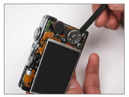
Remove the function buttons by sliding the spudger underneath the black rubber and lifting up.
