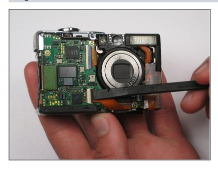
Remove the LCD cable by gently prying the hinge open with a spudger or your finger. The cable should easily slide out.
