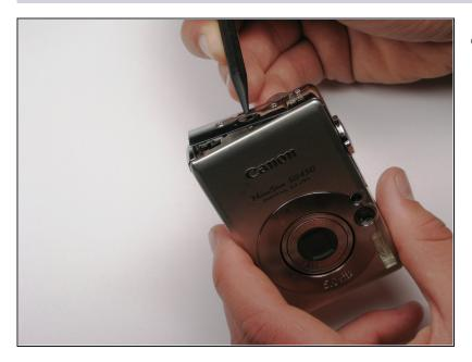
• Pull the lanyard mount off of the camera using a spudger or your fingers.
