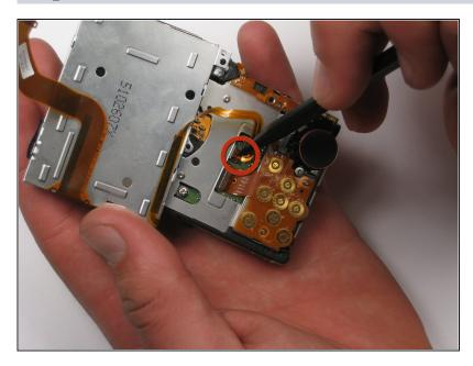
Pull the back light ribbon from it's socket to remove the LCD completely. There is a little hole you can stick the spudger into to help release the ribbon.
