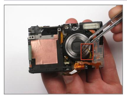
Grasp the plug that yellow and black wires are attached to, and gently remove. Tweezers are very helpful here.
