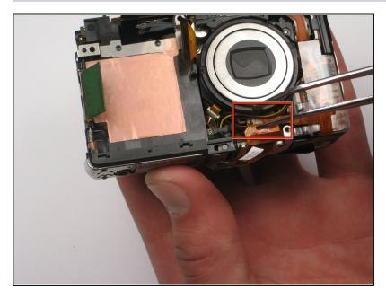
• Remove the orange ribbon from below the lens.
