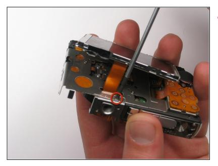
Remove the last screw holding the tripod mount to the case. The LCD ribbon threads under the mount, so upon reinstallation, the ribbon will need to be threaded through before the mount is reattached. Take note of the tripod mount orientation.
