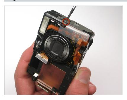
• Remove the side screw holding the flash bulb.
