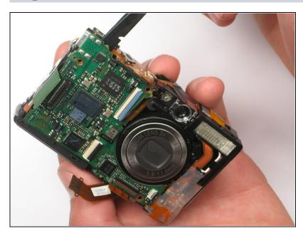
• Use the spudger to carefully remove the logic board from behind.
