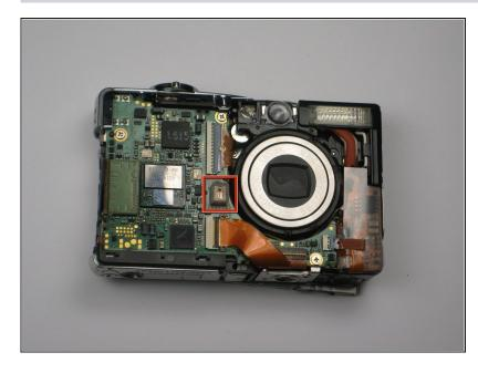
Remove the square, clear, rubber protector from the front of the logic board. This is not necessary to remove, but can easily fall off and get lost during later steps.
