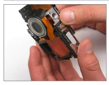
• Lift up the LCD screen WITHOUT removing it completely. The screen is still connected to the camera via a backlight ribbon underneath.
