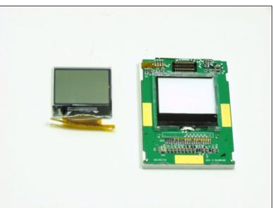
Pull the screen and the tape ribbon off the circuit board.
