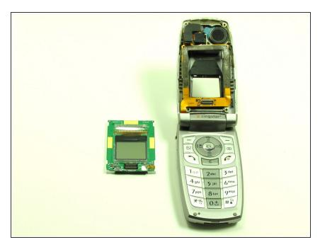
The outer LCD screen can be found on the circuit board, which is attached to the back of the inner LCD screen.
