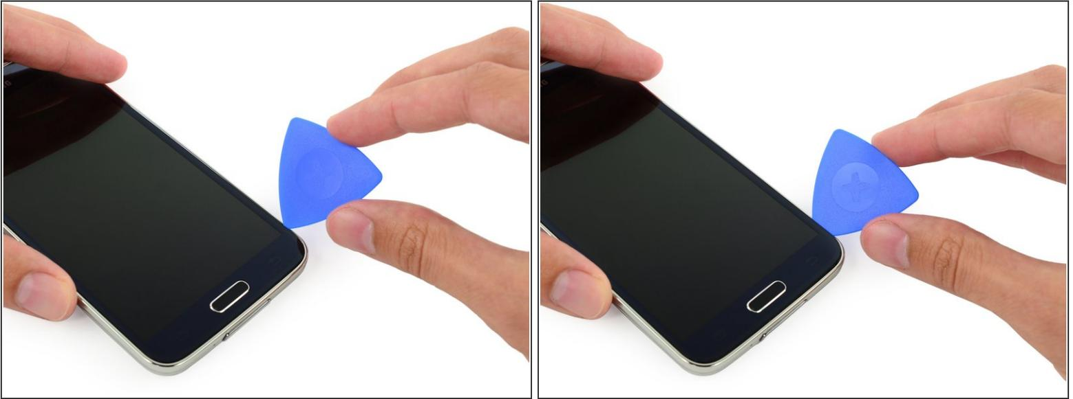
**i** In the following steps you will be using an opening pick to separate the adhesive securing the front panel glass. Only pry where directed. If you experience resistance, stop sliding the opening pick and reapply heat.
